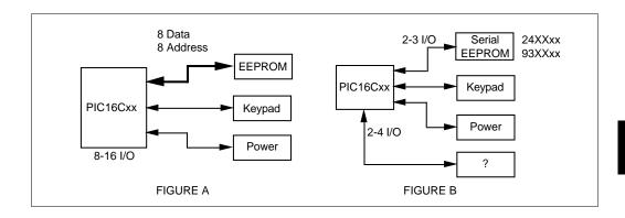
save power, board space, and cost, but they also offer the advantage of fewer I/O and consequently power in the embedded microcontroller because less I/O are needed to control the same functions. A typical embedded application is shown in Figure A, depicting a controller and several functions used in a personal communications device, such as a mobile or portable phone. The EEPROM stores speed dial and last number redial numbers, credit card numbers, ID numbers, and configuration parameters.
